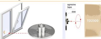
The transducer can be attached to the window pane or other smooth surfaces using the metal mounting disk.
