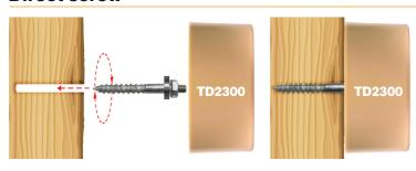
A double ended screw is provided in the supplied set. One end has machine screw threads for the transducer; the other has course, tapered threads to be used in such uniform materials such as wood, ply wood, studs, or wood beams.
