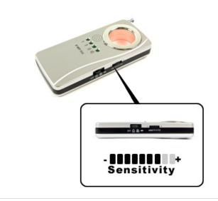
Electric wave sensitivity adjustment (may enhance sensitivity to pull large detecting range or depress sensitivity to shorten detecting range), so you can find out electric source even fast.
