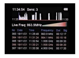
Graph Log Screen detecting pulsed signal
