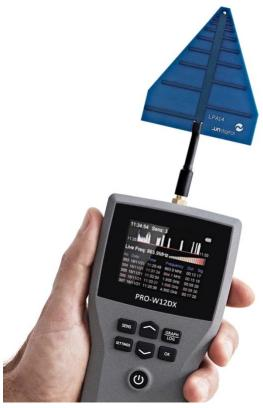
Detected signal strength is shown on a 20 element bar graph, enabling the user to locate the precise source of any detected signal. The frequency of the detected signal can be seen simultaneously and the new 'Livescan' software shows the detected live signal pattern graphically to help identify the signal type. This can be particularly useful when searching for pulsing or burst devices such as GPS trackers.
