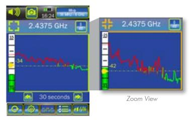
The signal strength histogram displays RF levels over user-selected time intervals ranging from 5 seconds to 24 hours. The adjustable trigger level provides audio, haptic, and visual alerts when RF levels exceed the threshold.
