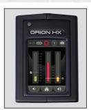
Tx and Rx graph displays power, 2nd and 3rd harmonic levels and touch screen trip and power level adjustments.
