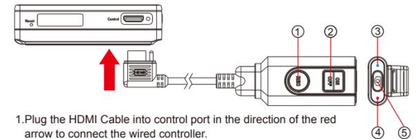
1. Plug the HDMI Cable into control port in the direction of the red arrow to connect the wired controller.
