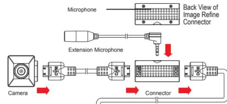
1. Connect camera to connector using required cable.
