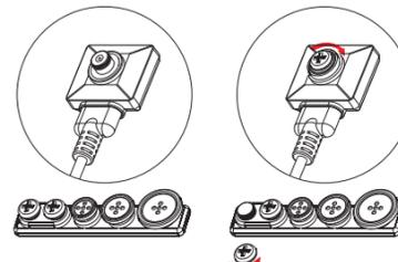
1. Take the lens cap off and unscrew the desired covert lens cap in counterclockwise direction from the set.
